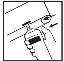
2. Press and hold the power switch; while the wheel is turning and the tachometer is measuring the selected function, the function will be indicated, and the unit of measure function will be flashing.
