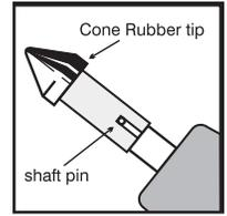
2. Bring cone into contact with the shaft. Apply only enough pressure to avoid slippage.
