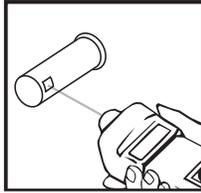
2. Aim the tachometer at the reflective tape from a distance of 5" (127 mm) to 20' (6.m).
