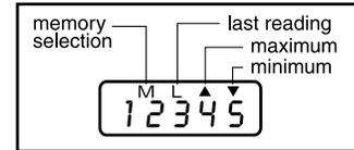
To fill all three memory spaces, unit must operate for about 5 seconds. If any of the above memory readings are missing, unit must operate a few seconds longer.
