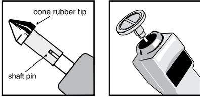
**CAUTION:** Do not attach master speed wheel on extension shaft. The wheel may slip off during measurement.
