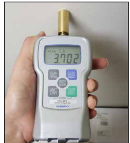
Performing Puncture Test on Drywall
